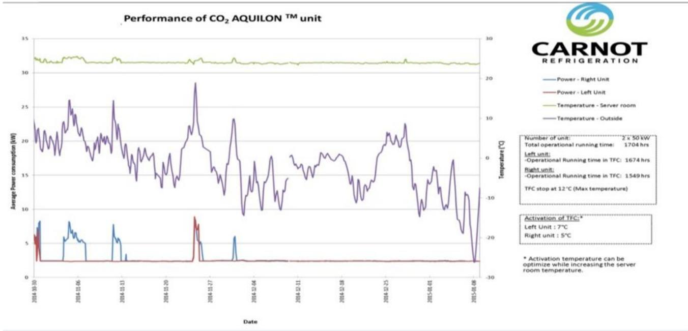
Graph above is showing period from November 2014 to January 2015. As it can be seen average running hours between two Carnot units in free cooling mode was 1,611 hours or 94.5% of total running hours
