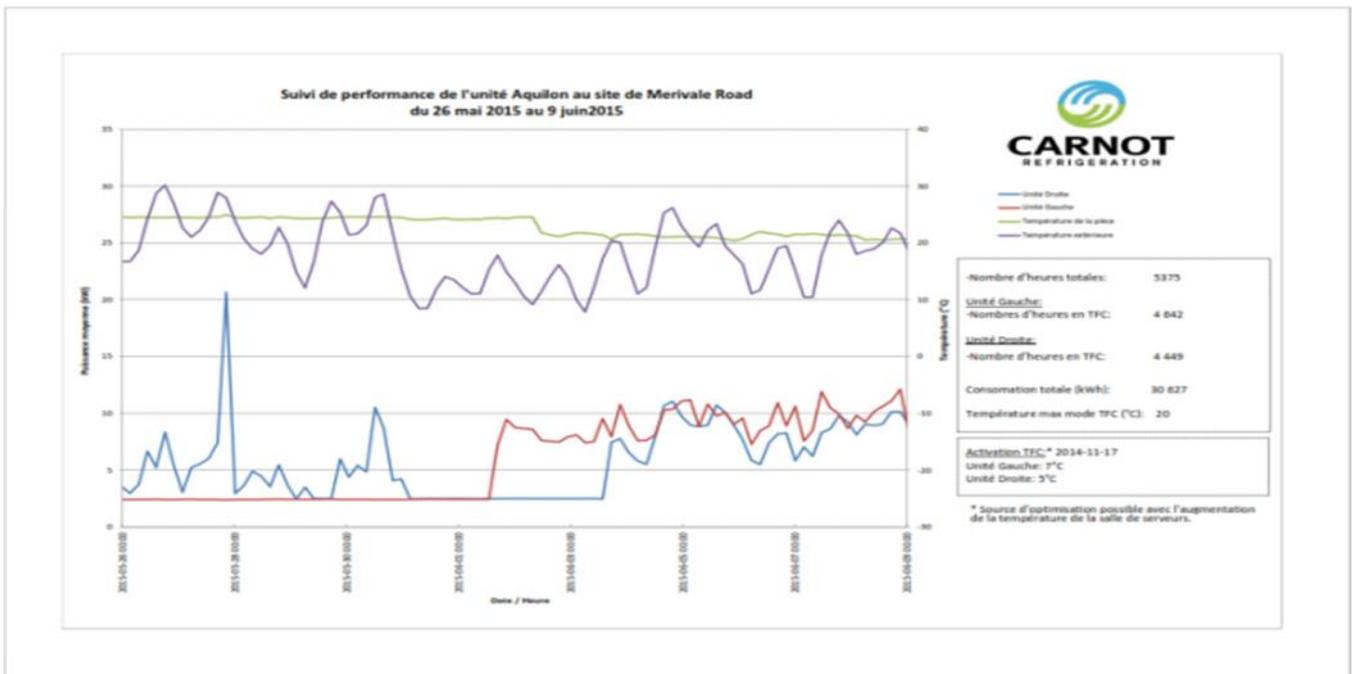
Graph above is showing period from May 26th to June 9<sup>th</sup> of 2015 As it can be seen average running hours between two Carnot units in free cooling mode was 4545 hours or 84.5% of total running hours
