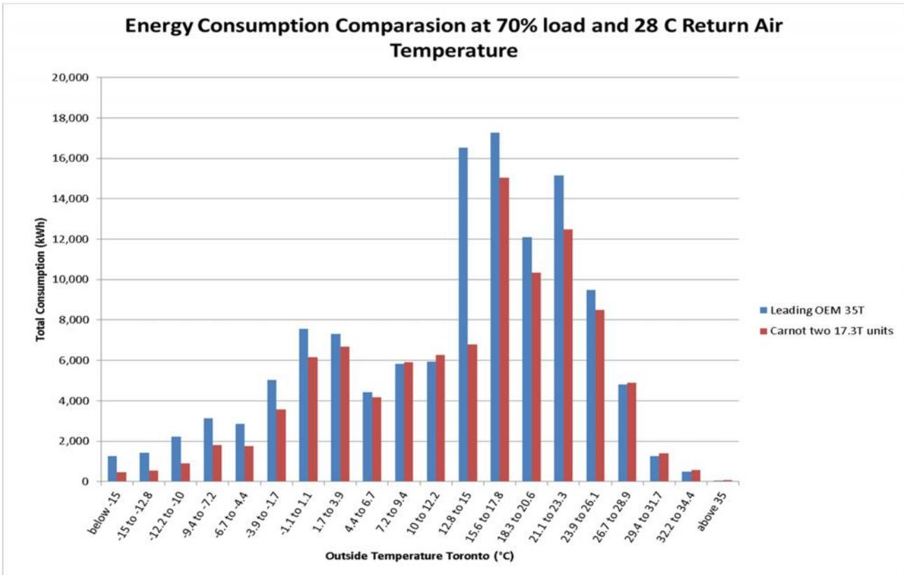
Graph above is showing Energy BIN comparison between 35TR Carnot and same capacity leading OEM unit. Note in particular BIN between 13 to 15 °C where Carnot is in total free cooling mode versus full mechanical or hybrid mode of leading OEM Data Center unit
