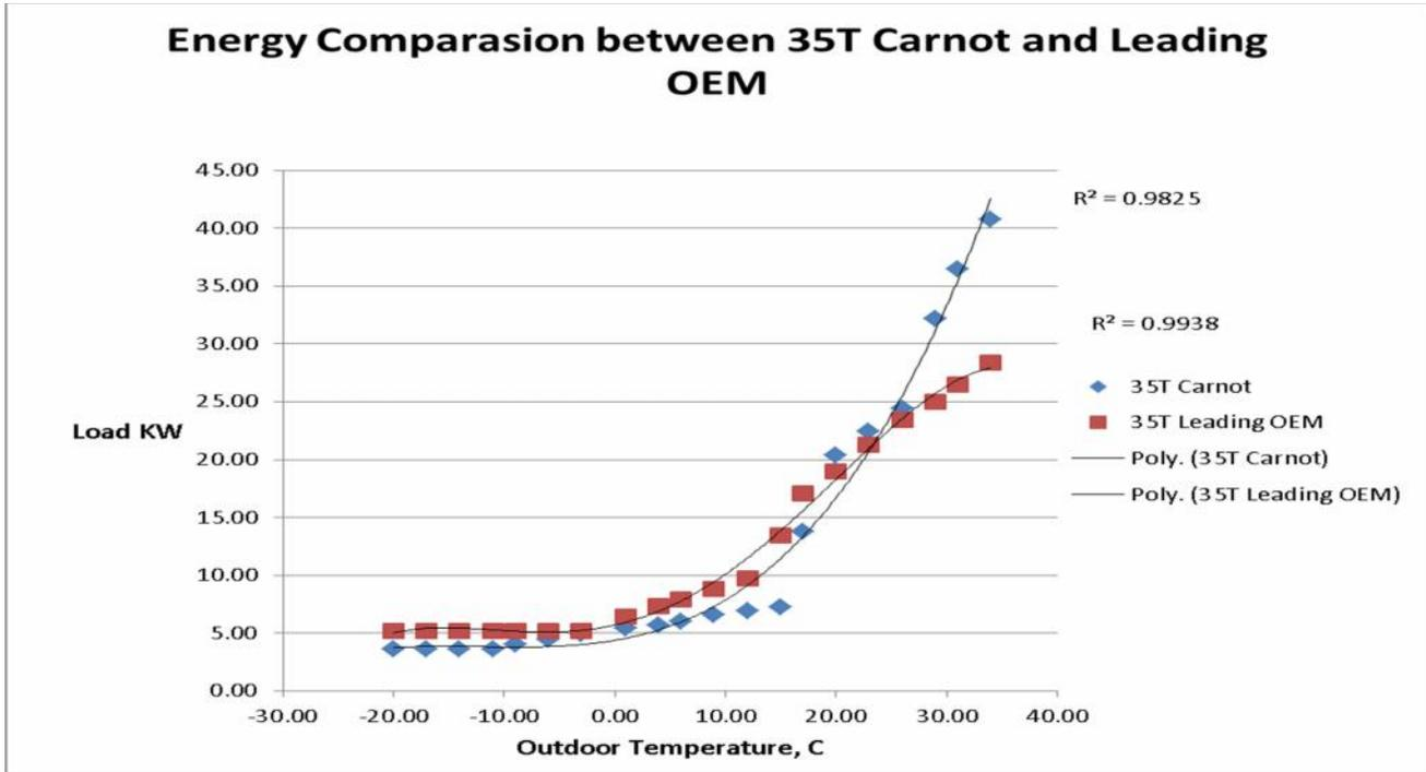
Graph above is showing BIN Energy Analysis between 35T Carnot unit and same capacity leading OEM Data Center unit. As it can be seen for temperatures below 7 °C both units are in a total free cooling mode with Carnot unit slightly more efficient. From 7 °C leading OEM unit is in the hybrid mode, while Carnot unit stays in the free cooling mode up to 18 °C. This represents 6360 hours or 72% of free cooling hours throughout whole year for Ottawa.
